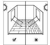
The floor should preferably be installed parallel to how the light enters the room (visually more attractive).
