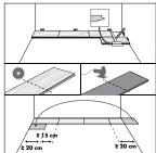
Of course you also need to saw the panels. To obtain a clean cut, the top surface should face down when you use a jigsaw, or circular handsaw and up when you use a handsaw or a crosscut saw. Ensure that the end joints of the panels in two successive rows are never in line. Always ensure that the joints are staggered by at least 15 cm.
