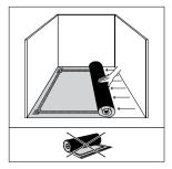
Remove any damp-open floor covering (carpet, needle felt, etc.) first. Damp-proof floor covering (PVC, linoleum, etc.) does not have to be removed. Always use an underlay. We recommend the use of Quick • Step® underlay.
