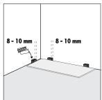
Put the plank with sawn off sides against the walls. Put spacers from the installation kit between the planks and the wall. This will ensure that your expansion joint is wide enough: 8 to 10 mm.
