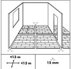
Large rooms must have expansion joints every 13 m breadthwise to the panels and every 13 m lengthwise. Expansion and contraction are linear, so the greater the surface area, the greater the tolerances need to be.
