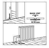
Wood is the main component of this Quick • Step® floor. Because room humidity can vary – for example, between summer and winter – it is vital that the floor is able to expand and contract. That's why you must leave an expansion joint on all sides of the floor of minimum 8 to 10 mm, also around pipes, under doors and at doorsteps. Remember that the floor may move in one direction.
