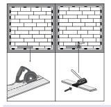
There must also be an 8 to 10 mm expansion joint between the last row and the wall. Keep this in mind when sawing the last row of panels.
