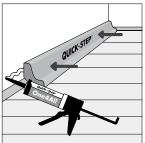
Install the skirting-board on the plastic foil that extends up the wall from under the floor. Never attach the skirting-board to the floor. This method allows the floor to expand and contract under the skirting-board.
