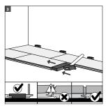
Tap the cross joint between these panels snugly together using the Uniclic tapping block. Make sure both panels are level on the subfloor and that you position the tapping block as indicated in the diagram to avoid damage.
