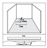
Make sure the floor base is flat. Any unevenness greater than 2 mm over the length of 1 meter must be smoothed out.
