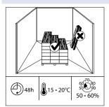
Let the planks acclimatize for 48 hours in the unopened packaging at the normal room temperature, in the middle of the room where the floor is to be installed. The ideal conditions are 15-20°C (59-68°F) at a relative humidity of 50-60%.
