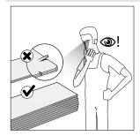
Inspect all planks in sufficient light before and during installation. Planks with visible defects must never be used.
