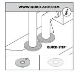
For a perfect finish around pipes, use Quick • Step® pipe covers or an elastic paste (Quick • Step® Kit).
