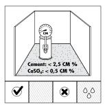
Fresh screed must dry for at least 1 week per cm thickness up to 4 cm and 2 weeks per cm thickness over 4 cm, with sufficient ventilation. For example, a 6 cm screed must dry for at least 8 weeks. For the thickness over 6 cm you must add 3 to 4 weeks. The moisture content must be less than 2.5% for cement-bound screed (CM method) and 0.5% for an anhydrite-bound screed.
