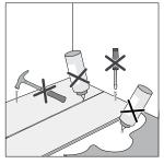
Uniclic® is a revolutionary system for installing floating laminate floors without using glue. The panels can be clicked together easily thanks to the ingenious shape of the tongue and groove.
