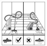
Dry maintenance is possible with Quick • Step® microfiber cloth or with a vacuum cleaner. Make sure it is equipped with soft wheels and a special parquet brush to avoid scratches on your floor. Never use a steam cleaner.
