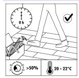
You can walk on the floor during and immediately after installation. Ensure that humidity in the room is always at least 50%. Use a humidifier if necessary.
